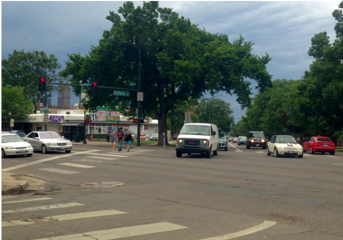
The odd angles created by the 5-way intersection at Colfax/Franklin/Park significantly increase the crossing distance for pedestrians.
