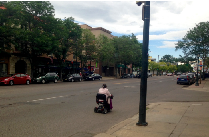
At intersections where streets north of Colfax do not align with streets south of Colfax (such as this one at Colfax and Marion) the curb ramps on one side of Colfax are often not aligned with curb ramps on the other side, causing wheelchair users to travel in the street when crossing at these locations.
