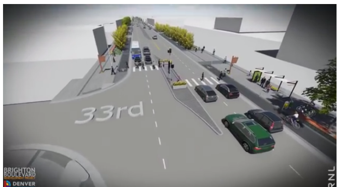
Planned mid-block crossing at 33 rd Street and Brighton Boulevard. Image source: City and County of Denver.
